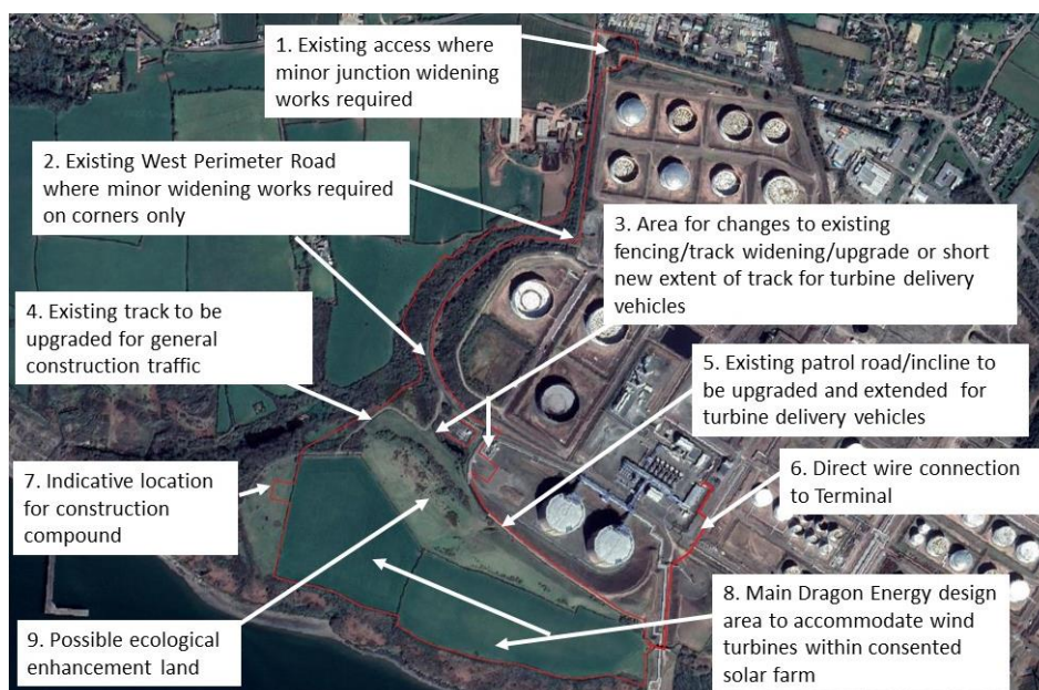
Figure 3.1 Site location plan annotated with key components of the Proposed Development
