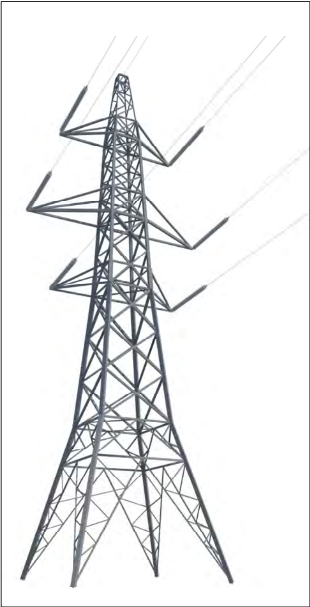
Component parts of 132kV steel lattice tower L7: Terminal tower
