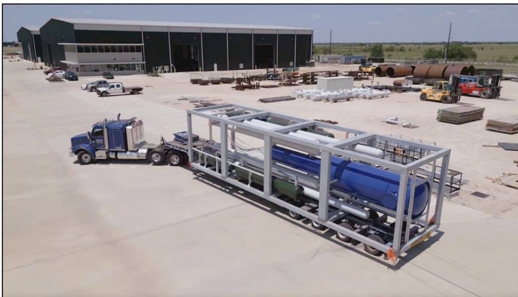
Figure 5.3 –Abnormal Load Vehicle and PWR-20 Module (Last Energy, 2024)
